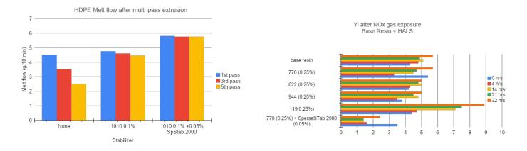
The graphs above show the retention of properties and color with a small addition of SperseStab 2000 to a traditional AO package.
